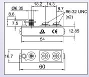
Screw adjust with mounting bracket
